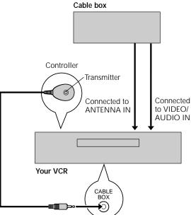
This procedure is required if you receive your TV channels through a cable box (descrambler). The Controller allows the VCR to automatically switch the cable box channel during timer-recording. The Controller is effective for recording shows that have been programmed using G-CODE ( pg. 40) or On-Screen Timer Programming ( pg. 42).
